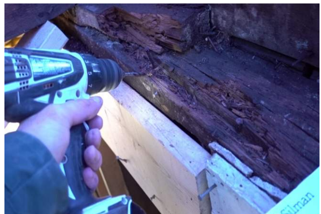
Figure 24 Close up of top of west wall being drilled for resistance.
