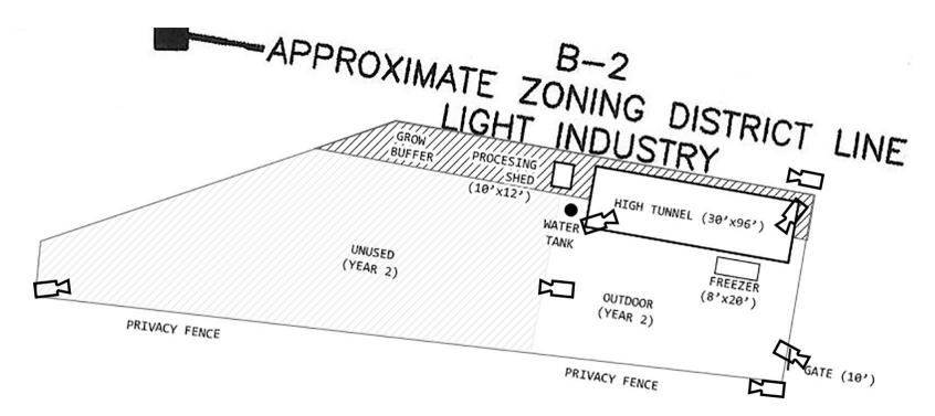
Security cameras will be installed as shown.
